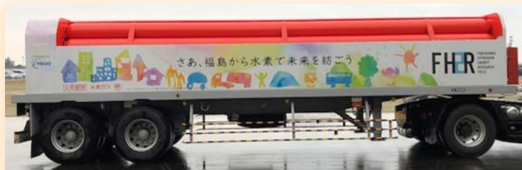
鱼雷车（压缩氢）约2700m 3 -H 2
